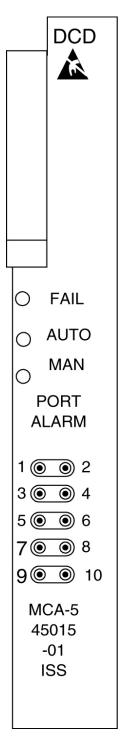
Figure 139: Holdover Clock MCA Card LEDs
