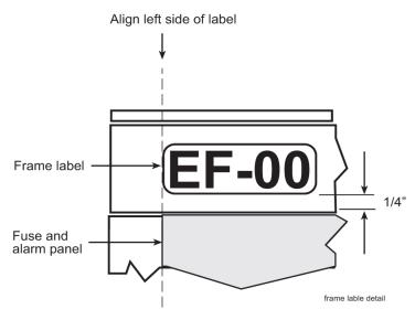
Figure 33: Frame Label Location - Detail
