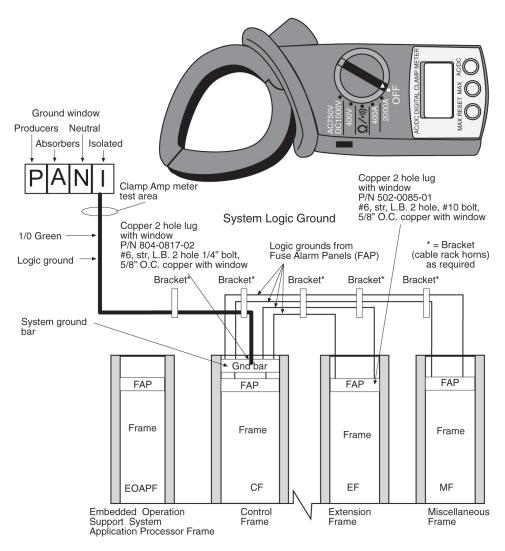
Figure 52: System Logic Grounding
