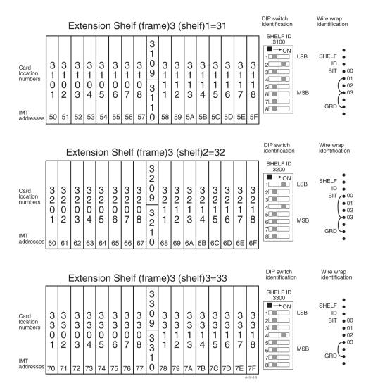
Figure 65: Extension Frame EF-01 Numbering Plan
