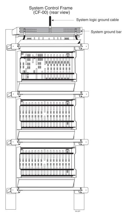
Figure 53: System Logic Ground Bar and Cable
