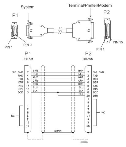
Figure 238: Terminal/Printer Cable
