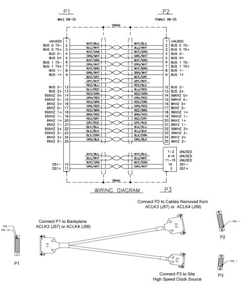
Figure 104: High-Speed Master Timing Adapter Cable (P/N 830-0846-01)
