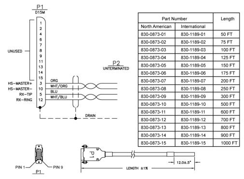
Figure 215: Master Clock Cable (BITS/High-speed)
