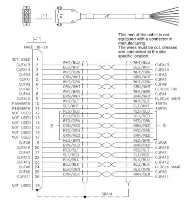
Figure 205: External Alarm Cable (Custom)
