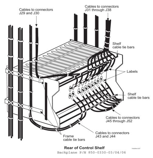
Figure 77: Interface Cable Routing, Control Shelf
