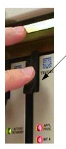
Push in the inject/eject clamps to lock the card in place.
