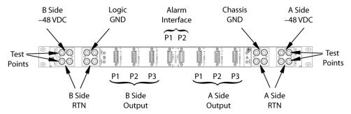
Figure 49: 1U Fuse and Alarm Panel Rear (P/N 870-2804-01)
