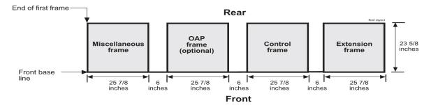
**Figure 14: Typical Frame Layout**
