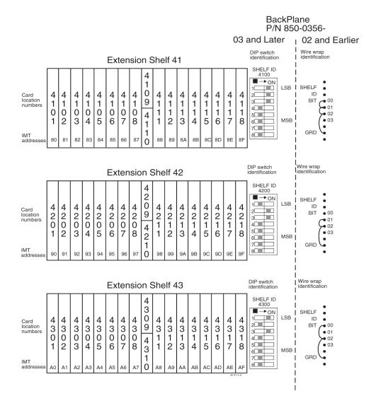
Figure 66: Extension Frame EF-02 Numbering Plan
