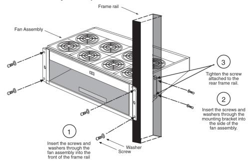
Figure 94: Installing Fan Assembly
