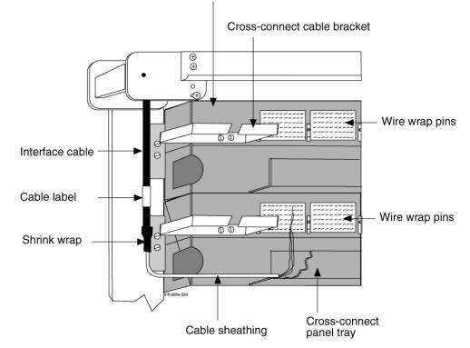
Figure 73: Interface Cable Cross-Connect Panel Connection
