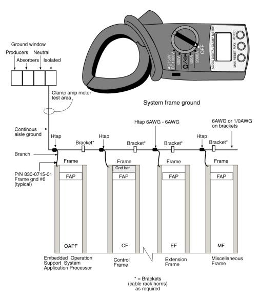
**Figure 51: System Frame Grounding**
