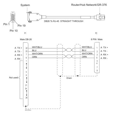
Figure 236: Straight Through Patch Panel Cable
