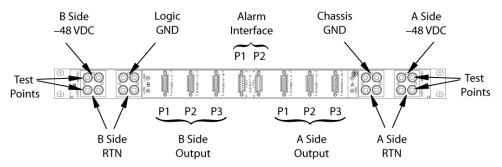
Figure 37: Fuse and Alarm Panel Rear (P/N870-2804-01).
