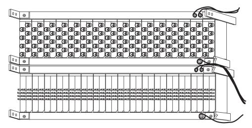
Rear 120 ohms to 75 ohms converter
