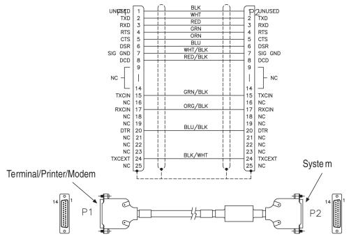
Figure 218: Modem/Terminal Cable
