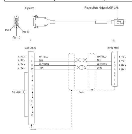
Figure 193: Crossover DCM Patch Panel Cable
