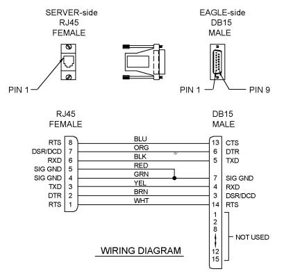
Figure 241: Terminal/Server Serial Port Adapter, MRV (P/N 830-0915-02)
