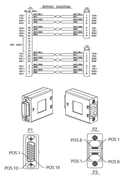
Figure 200: DB26 Male to Dual RJ45 Adapter
