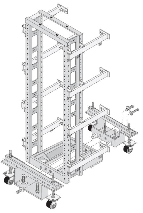
Figure 13: Heavy Duty Frame with Dolly
