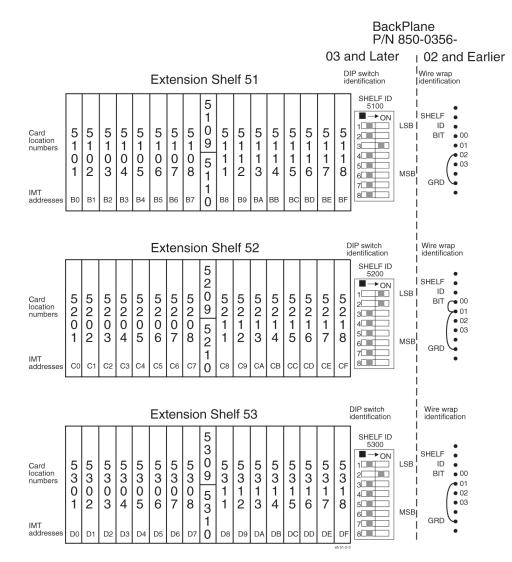
Figure 67: Extension Frame EF-03 Numbering Plan
