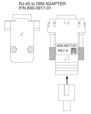
Figure 228: RJ 45 to 9 Pin Adapter
