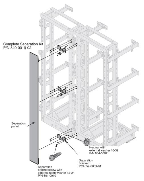
**Figure 25: Unit Separation Bracket Installation**
