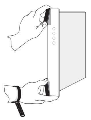
Figure 4: Removing a Card
