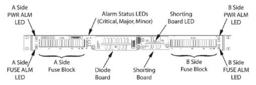
Figure 36: Fuse and Alarm Panel - Front View (P/N 870-2804-xx)
