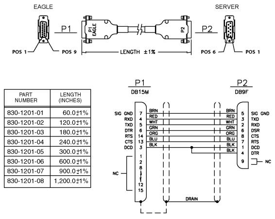
Figure 239: Terminal Server Serial Cable with Flow Control (P/N 830-1201-xx)
