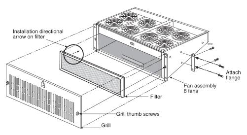
Figure 93: Fan Assembly with Grill and Filter
