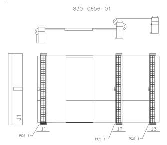
Figure 206: Fifty Position/Hard Drive I/O Cable
