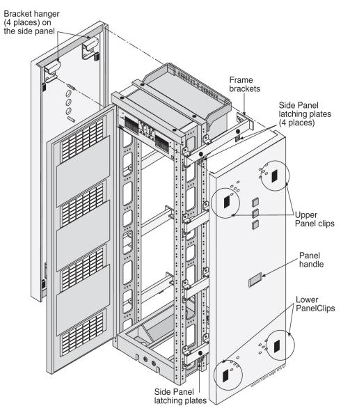
**Figure 24: Heavy Duty Frame Panels**
