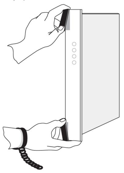
Figure 5: Removing an EAGLE card
