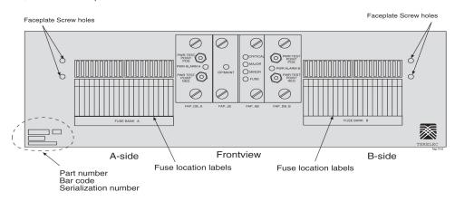
Figure 42: Fuse and Alarm Panel (P/N 870-1606-xx/870-2320-xx) Front
