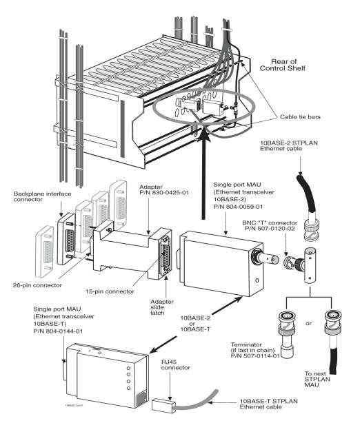
Figure 75: LAN Ethernet Cable Installation
