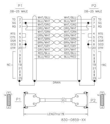
Figure 221: Null-MODEM for Terminal
