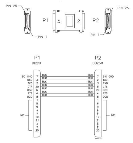
Figure 233: Serial Interface/Modem Adapter
