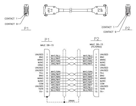
Figure 207: Filter Rack Alarm Cable
