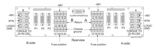
**Figure 116: Holdover Clock FAP Connections**
