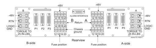
Figure 50: 3U Fuse and Alarm Panel Rear (P/N 870-2320-03))
