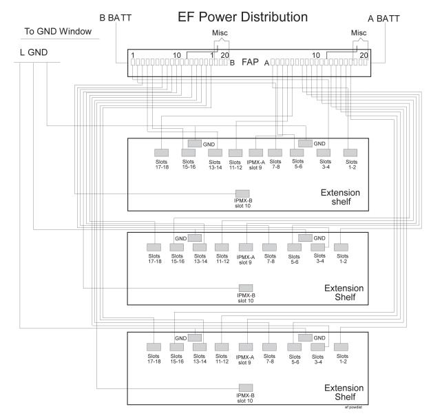
Figure 62: Extension Frame FAP (P/N 870-0243-08 and P/N 870-1606-xx)
