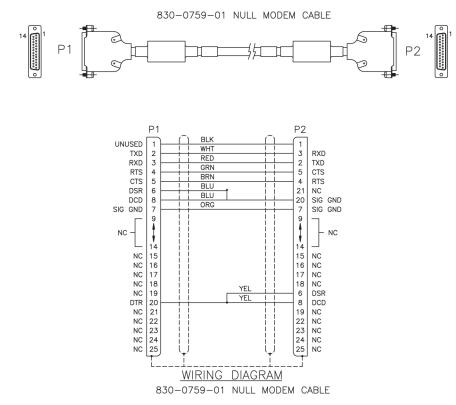
Figure 220: Null Modem Cable
