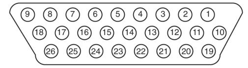
Figure 180: Extension Shelf Interface Connector
