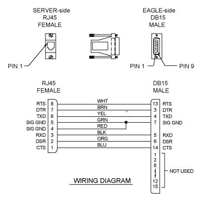
Figure 240: Terminal/Server Serial Port Adapter, NTW (P/N 830-0915-01)
