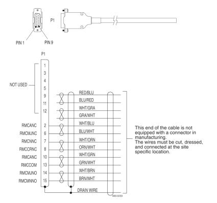
Figure 225: Remote Maintenance Center Cable
