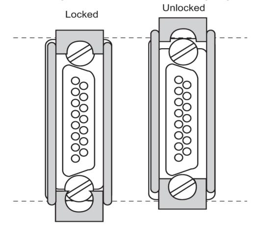
Figure 74: Adapter Slide Latch
