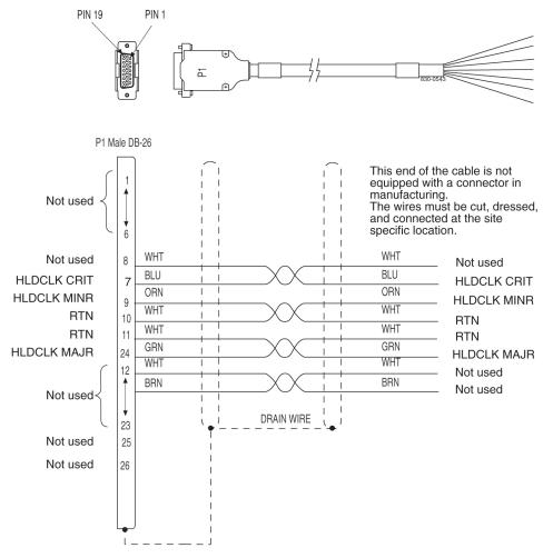
Figure 185: Holdover Clock Alarm Cable
