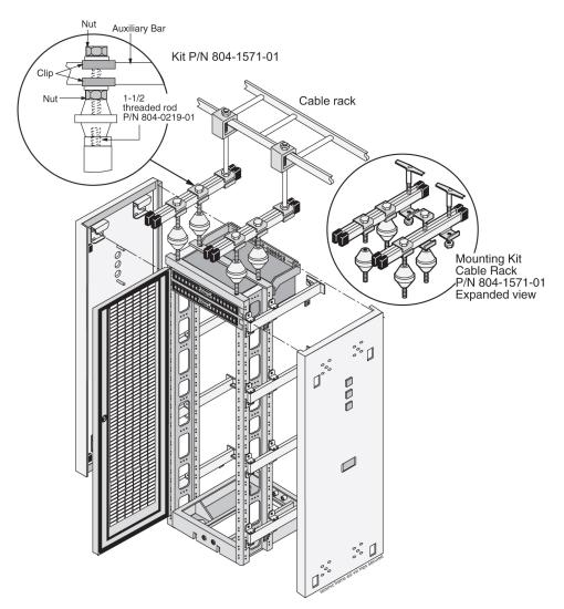
Figure 23: Heavy Duty Frame Installation With Cable Rack
