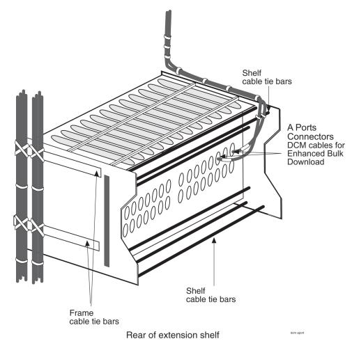
Figure 76: E5-ENET/E5-ENET-B Family Cabling, Enhanced Bulk Download
