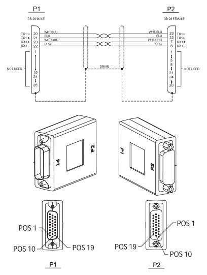
Figure 201: DB26 Male-to-DB26 Female Adapter
