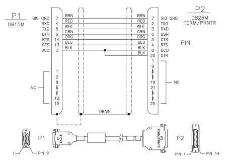
Figure 217: Man-Machine Interface Port Cable
