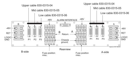
**Figure 115: Holdover Clock FAP Connections**
