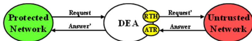
Figure 14: Diameter Topology Hiding Trigger Points: Protected-to-Untrusted Transactions
