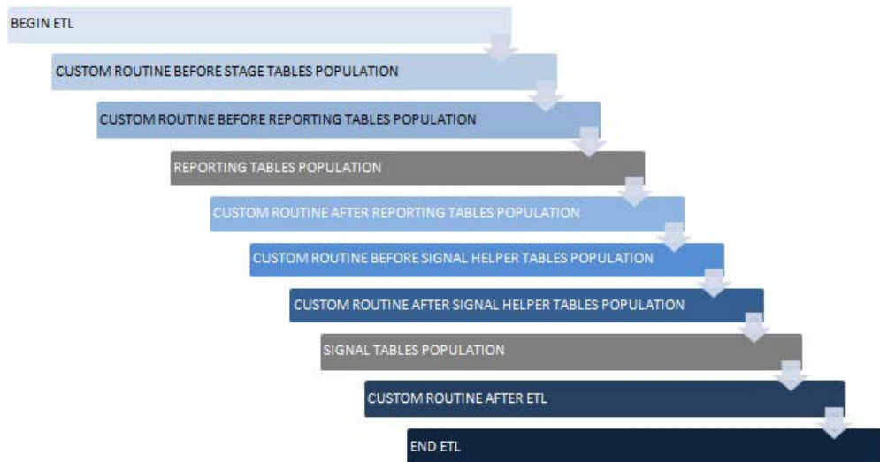
Figure 2-3 Sequence of ETL Hook Execution
