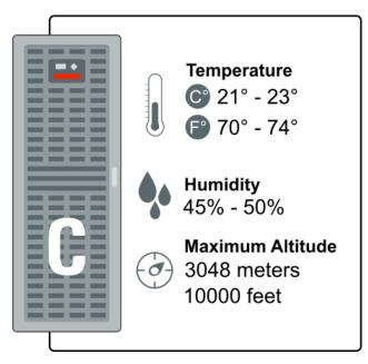
The following table lists the temperature, humidity and altitude requirements for Exadata Cloud Machine.
