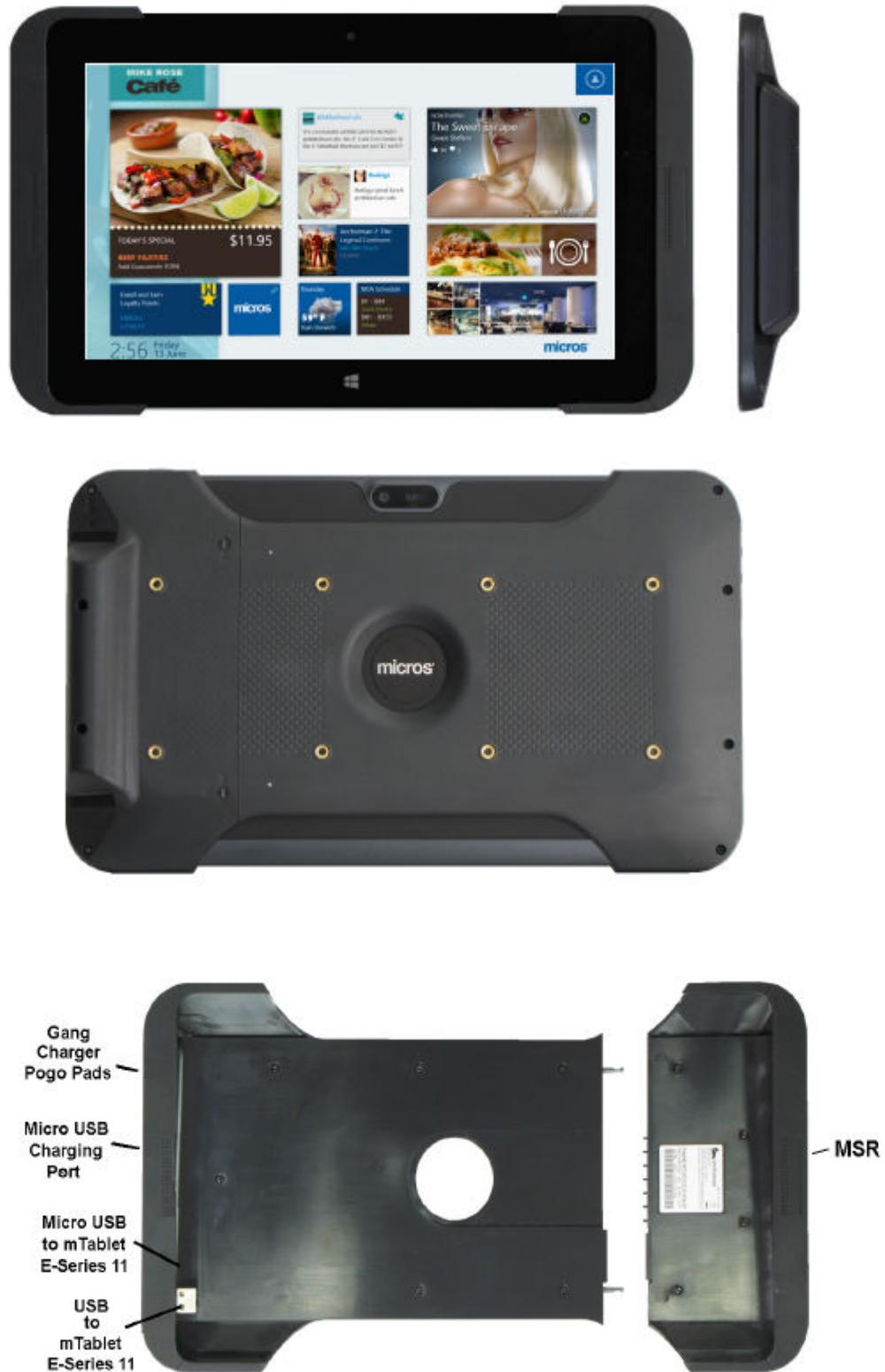
Figure 7-4 MICROS Tablet E-Series 11 with MSR Sleeve Features and Connectors
