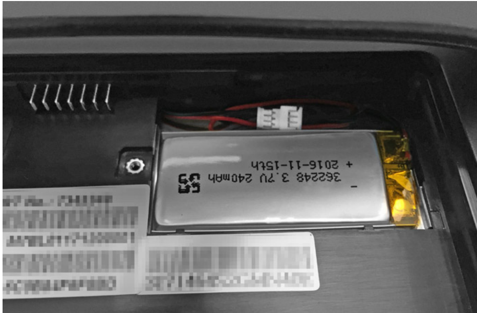
Figure 5-8 The Bridge Battery in the Battery Compartment
