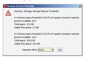
The Suppress Alerts list at the bottom of the dialog box functions identically to the other warning and error dialog boxes. In the previous figure a warning was issued to notify the operator that the DISK\_MIN\_SPACE\_THRESHHOLD\_PERCENT was reached.
