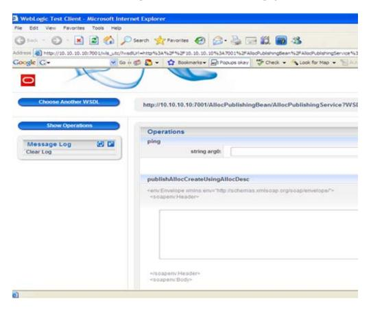
Modify the SOAP request body as needed. Click on the method required to invoke the corresponding method of the Web service. Once the method call is complete, the SOAP response will display in the same page.
