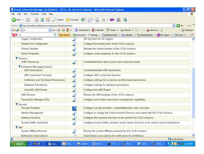
On the Security Providers screen, select the **Instance Level Security**.
