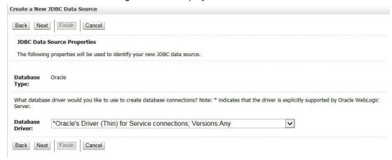
8. Select the Database Driver 'Oracle's Driver(Thin) for Services connections; Versions: Any'.
