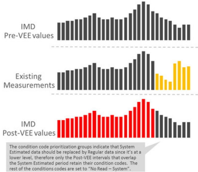
Example 4: Partial replacement of regular data with outage data based on condition range prioritization
