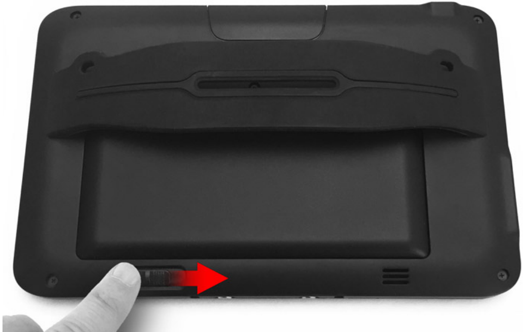
Figure 7-2 Removing the MICROS Tablet 720 Main Battery
