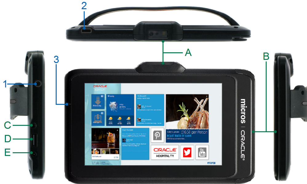
Figure 1-4 The Features of the Oracle MICROS Tablet 720 — Front and Side View
