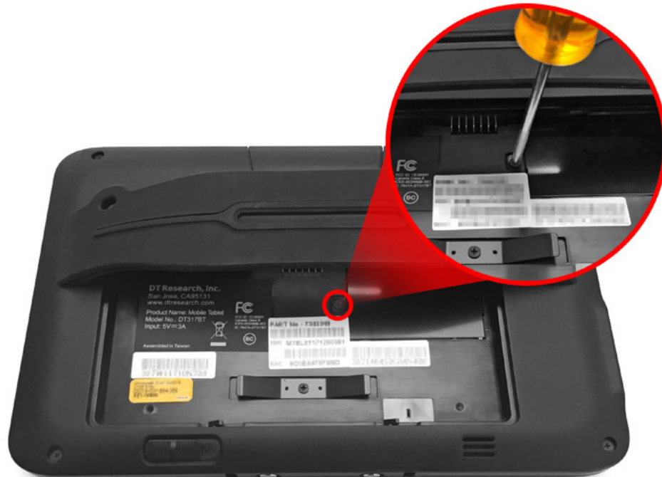
Figure 7-3 Removing the Bridge Battery Cover
