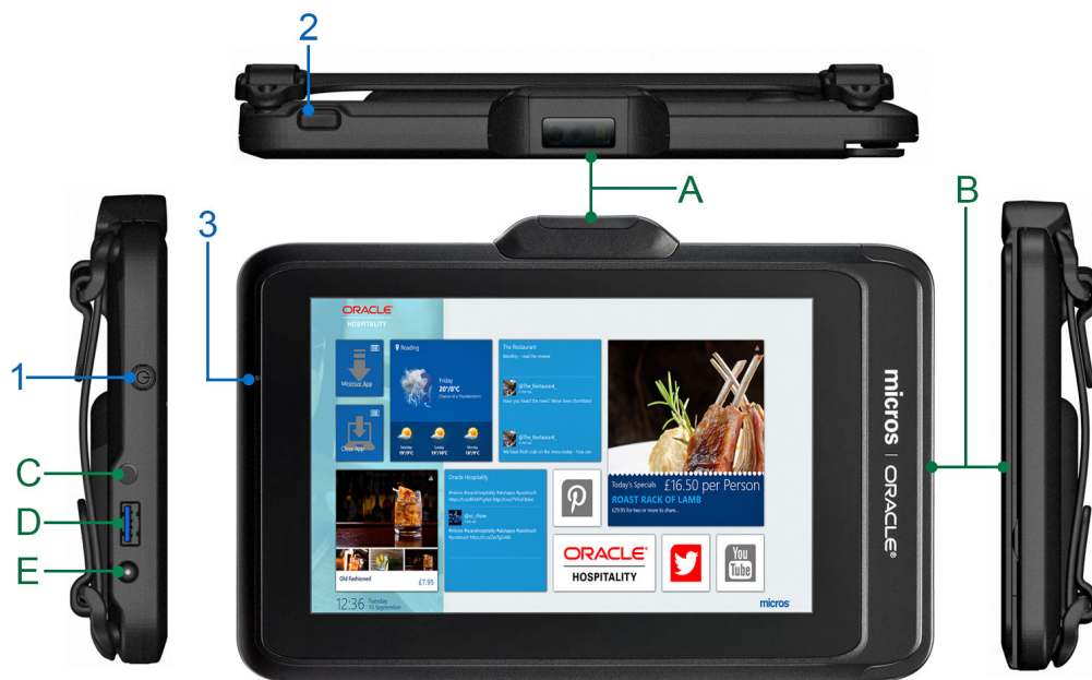
Figure 1-2 The Features of the Oracle MICROS Tablet 721 — Front and Side View
