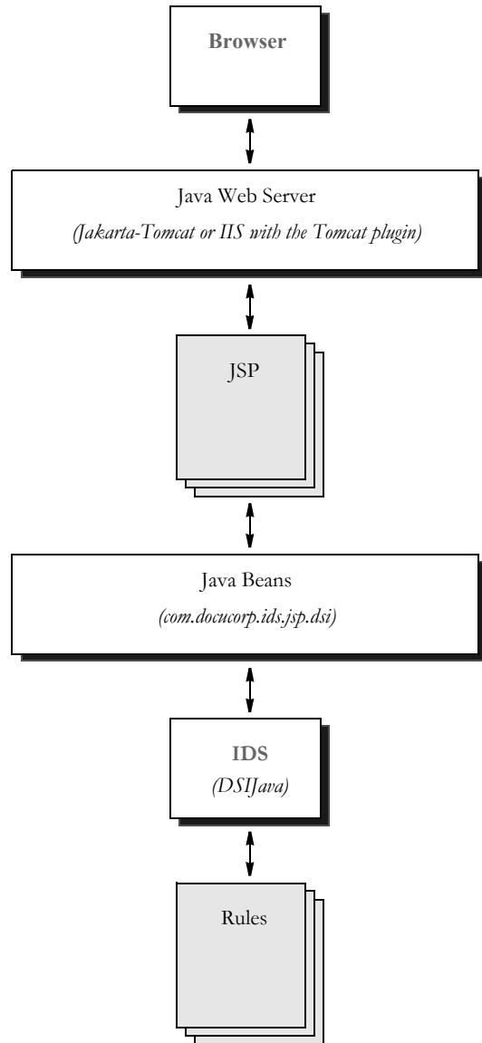
The name *REQTYPE* is reserved for the request type to the IDS rule. Once the request name/value has been passed to the dsi JavaBean, ProcessRequest is called to send the name/value and request type to the IDS rules.
