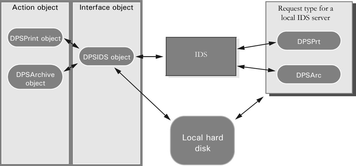
This illustration shows how it works with IDS running on a different machine:
