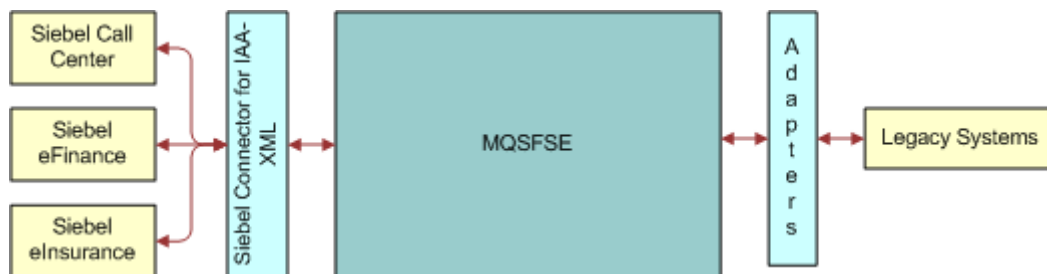
Figure 4. Integration Between Siebel Applications and MQSFSE
