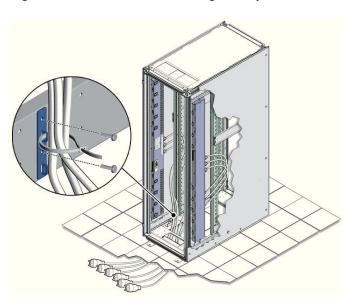
Figure 6-8 Power Cord Routing Example
