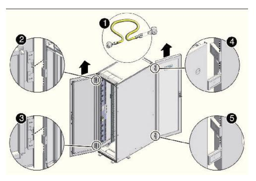
Figure 7-2 Removing the Rack Doors
