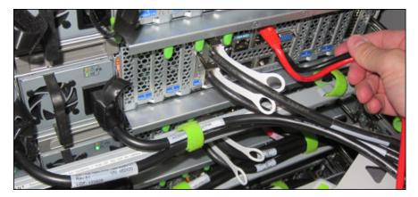
Route the cables through the CMA and secure them with hook and loop straps on both sides of each bend in the CMA.
