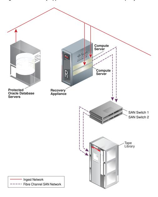
Figure 3-4 Recovery Appliance Connection to an Oracle Tape System
