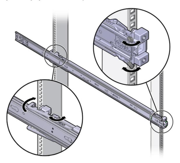
Figure 7-5 Aligning the Side-Rail Assembly With the Rack
