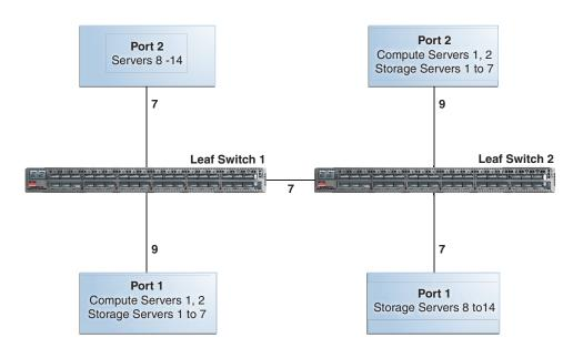
Figure G-2 In-Rack Connections Between the Servers and the Leaf Switches
