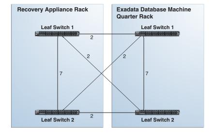
Figure 9-1 Recovery Appliance Connected to an Exadata Quarter Rack
