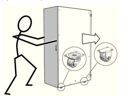
Figure 6-2 Carefully Push ZDLRA Rack from Behind
