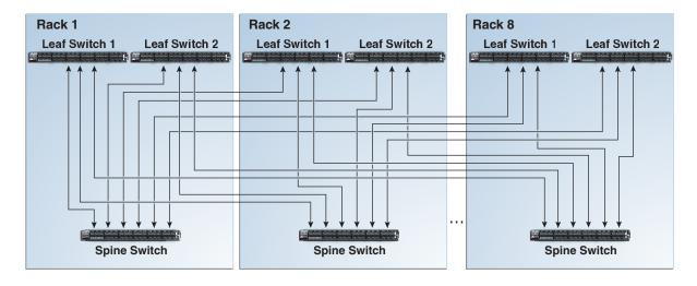
Figure G-4 Connecting Switches Across Eight Racks
