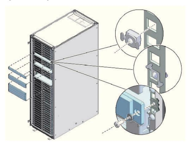
Figure 7-3 Removing the Filler Panels
