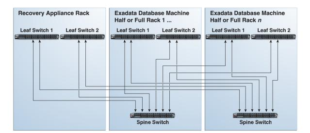
Figure 9-3 Recovery Appliance Connected to Multiple Exadata Racks
