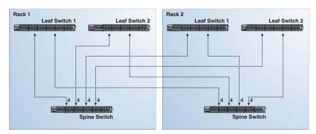
Figure G-3 Connecting Switches Across Two Racks
