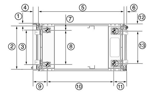
Figure 6-3 Location of Leveling Feet on ZDLRA Rack
