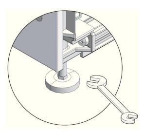
Figure 6-4 Securing ZDLRA Rack Using the Leveling Feet
