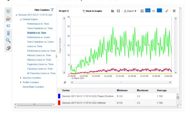
Figure 4-21 Statistics vs. Time Custom Graph with Zoom Mode On
