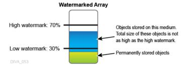
The following figure represents a watermarked disk array with permanently stored objects with a total size that is less than the Low Watermark, and temporarily stored objects with a total size that has reached the High Watermark level. In this figure the temporary objects have now reached the High Watermark, and will be removed using one of the two methods available (Last Access Time or Largest Object Size) until the level reaches the Low Watermark.
