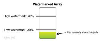
The following figure represents a watermarked disk array with permanently stored objects with a total size that is less than the Low Watermark, and temporarily stored objects with a total size that is higher than the Low Watermark:
