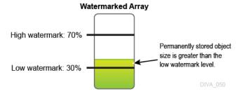
The following figures characterize a typical Watermarked Medium (watermarking set to Yes) and illustrate how watermarking ensures the medium does not reach full capacity.
