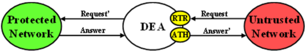
Figure 10-3 Diameter Topology Hiding Trigger Points: Untrusted-to-Protected Transactions
