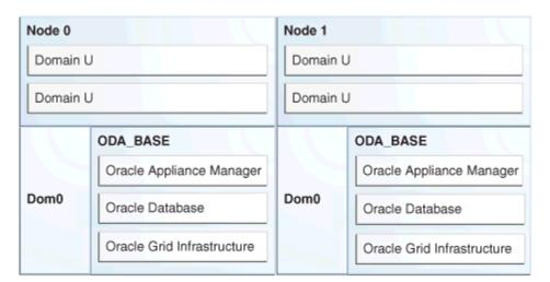
Figure 12-1 Oracle Database Appliance Virtualized Platform Architecture
