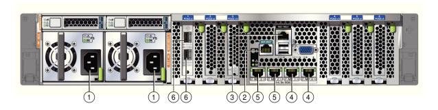
Table 3-1 Location of Network Ports and Power Cabling for Oracle Database Appliance
