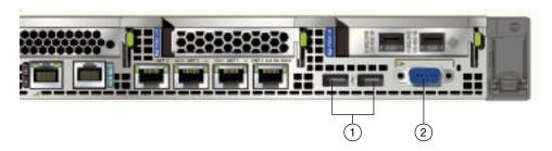
In the figure, callout 1 identifies the ports for the keyboard and mouse. Callout 2 identifies the monitor port.
