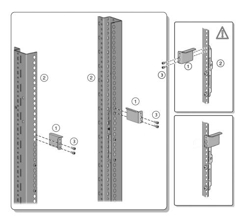
Before tightening the screws, slide the brackets [1] up as far as they will go. The holes on the brackets are oval-shaped so they can move up and down when the screws are loose.
