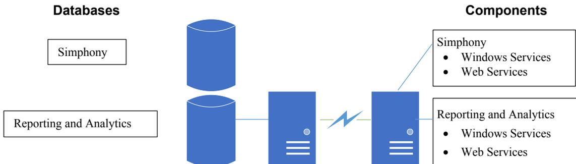
Figure 1-4 Example of Application Components and DBs on Separate Servers
