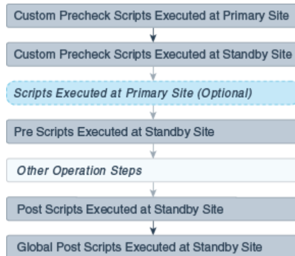
Figure 2-5 Execution Sequence of Scripts for Failover Operation
