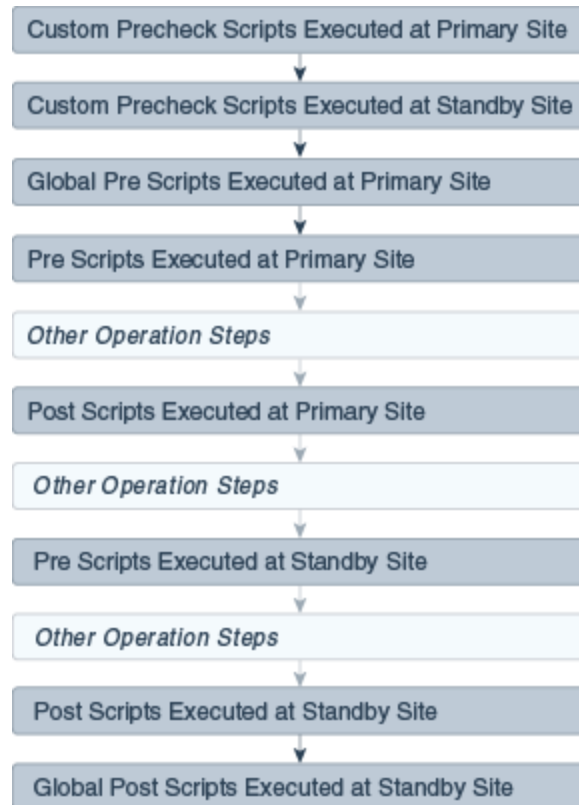
Figure 2-4 Executing Sequence of Scripts for Switchover Operation
