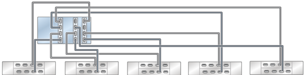
FIGURE 103 Standalone ZS4-4 controller with three HBAs connected to six DE3-24 disk shelves in six chains
