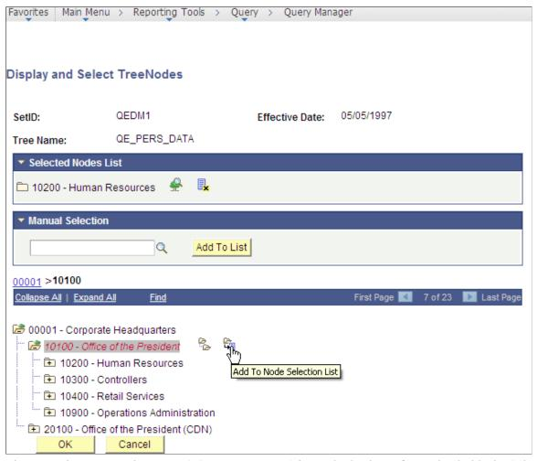
The Tree Viewer secondary page (PSTREEVIEWER) in Method B has a frame that holds the Selected Nodes List with action buttons associated with each selected node. This page is used to select the set of nodes, return them to the calling application (Query Manager), and use the list of nodes as Query criteria.
