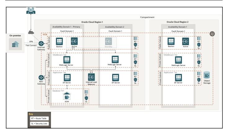
The deployment architecture consists of two Availability Domains used for OFSAA and WebLogic Server in the same Oracle Cloud Infrastructure (OCI) Compartment. Oracle Identity Cloud Service (IDCS) can be used to log in. The Load Balancer (LB) redirects the request to respective compute.
