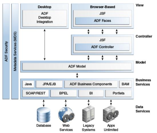
Figure 1-1 ADF Architecture with ADF Model
