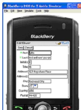
Figure 6–3 Difficulty Displaying Input Fields and Labels with Font Size at 6 pt.
