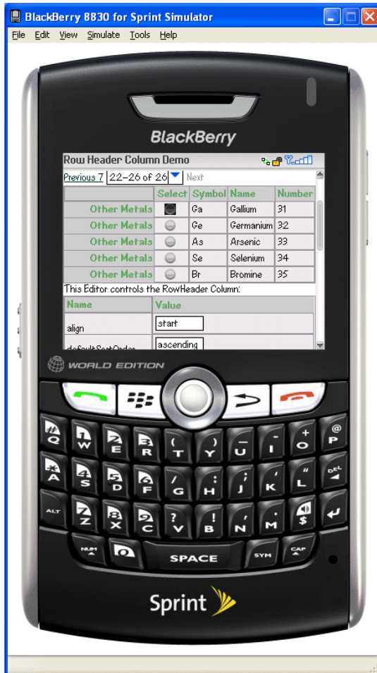
Figure 2–11 Testing an ADF Mobile Browser Application on a BlackBerry Smartphone Simulator
