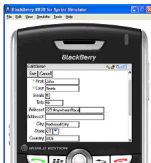
Figure 6-1 Application Display Using the Default Font Size of 6 pt.
