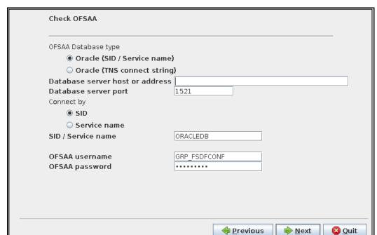
5. The installer checks for the OFSAA database when the database details are entered.
