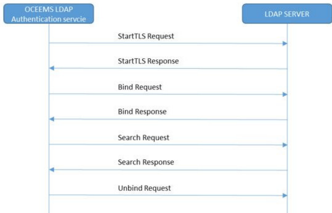
Figure 4-1 Sample Call Flow for LDAP Authentication
