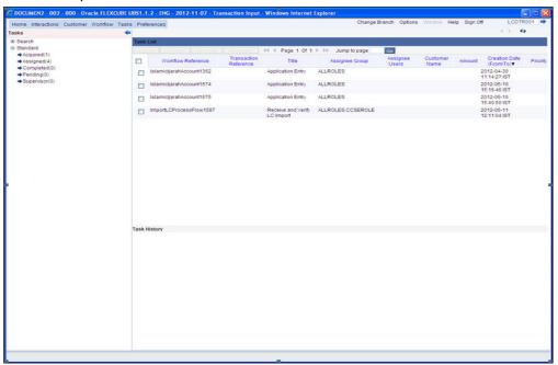
All tasks that have been successfully completed are listed in the right side of the screen. Select the checkbox against your 'Workflow Ref No' and click 'Acquire' button at the top of the screen to acquire the next stage of the task.
