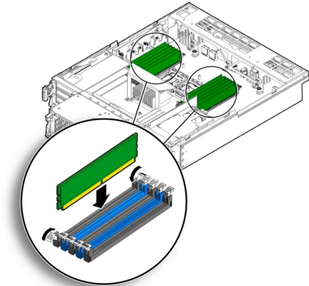
5. **Push the DIMM into the connector until the ejector tabs lock the DIMM in place.**
