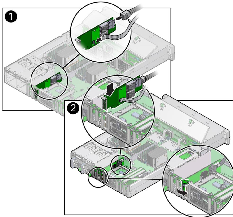
11. Insert the SAS HBA card into PCIe slot 3 [2], and rotate the PCIe locking mechanism to secure the PCIe HBA card in place [1].
