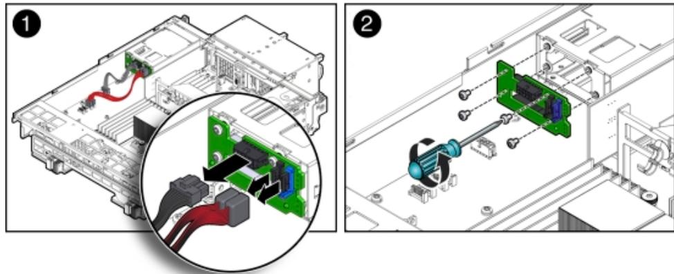
**b. Remove the four Phillips screws that secure the boot disk backplane to the rear-mounted disk drives assembly and remove the backplane [2].**
