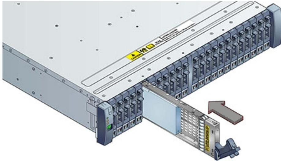
4. **Once installed, the system should automatically detect and use the replacement drive. Ensure that the green OK indicator for the replacement drive lights to show that the drive is ready.**
