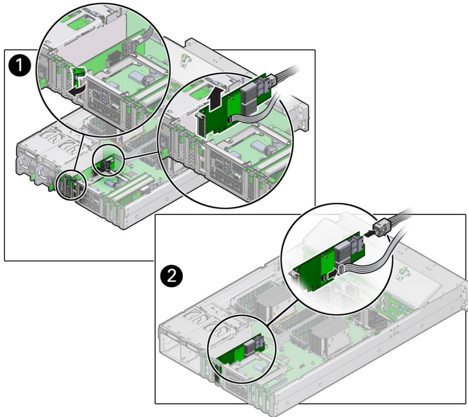
5. **Disconnect the super capacitor cable and the SAS cables from the SAS HBA card [1].**
