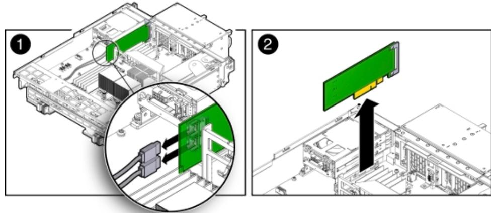
**b. Disconnect the data cables from the PCIe card [1].**
