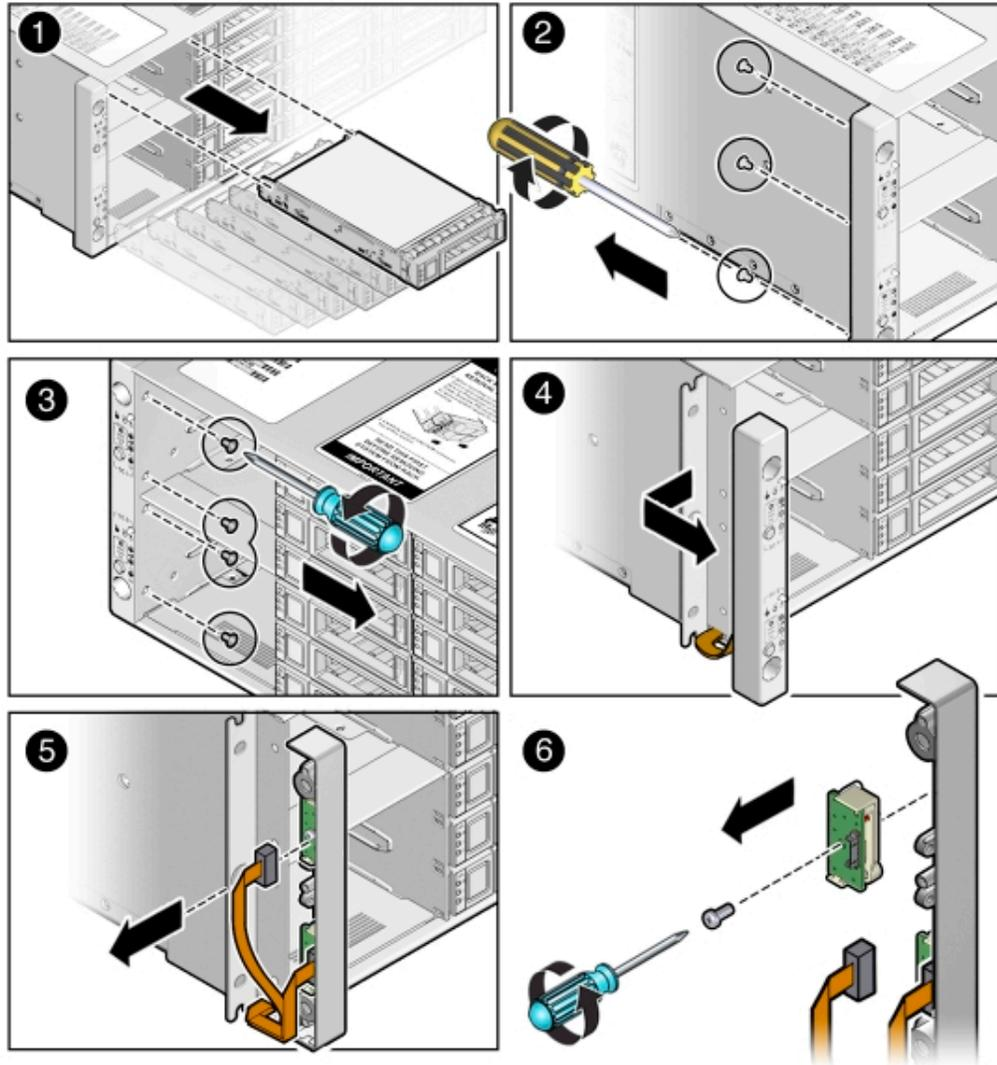
7. Remove the screw that holds the indicator panel to the ear bezel [6].
