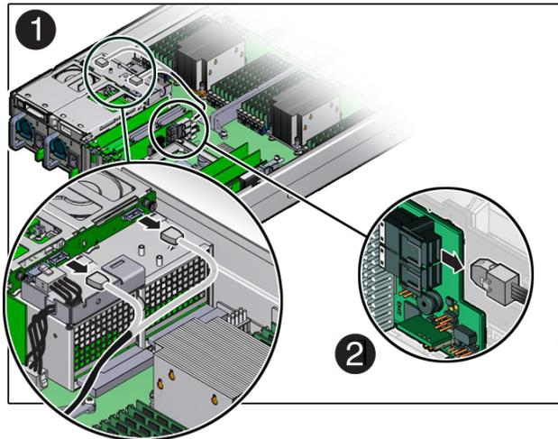
4. Install the replacement SAS cable to the rear disk drive backplane [1] and the SAS card [2].
