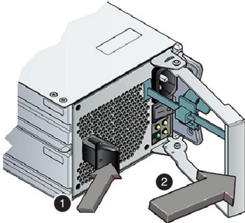
4. **Open the lever/ejection arms on the replacement power supply.**
