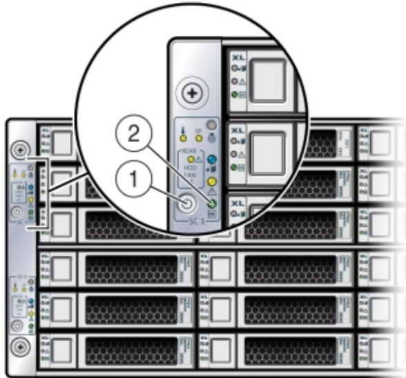
On the server node, the green Power/OK LED [2] blinks while the server node is booting, and remains steady on when the server node is operational.
