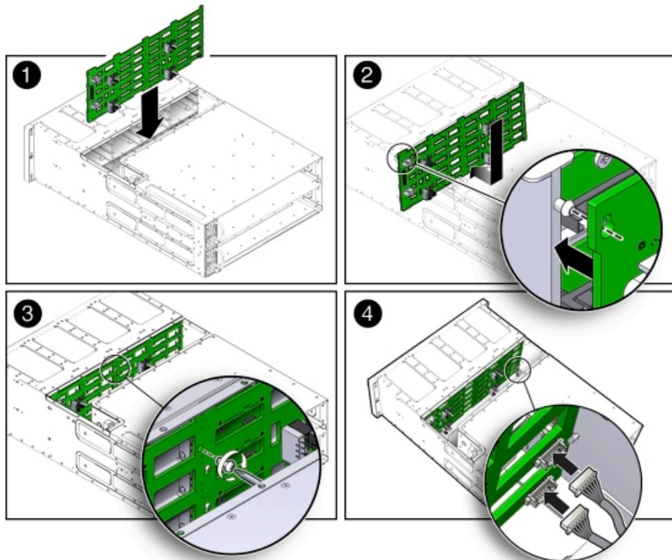
2. **Install the power distribution board into the system.**
