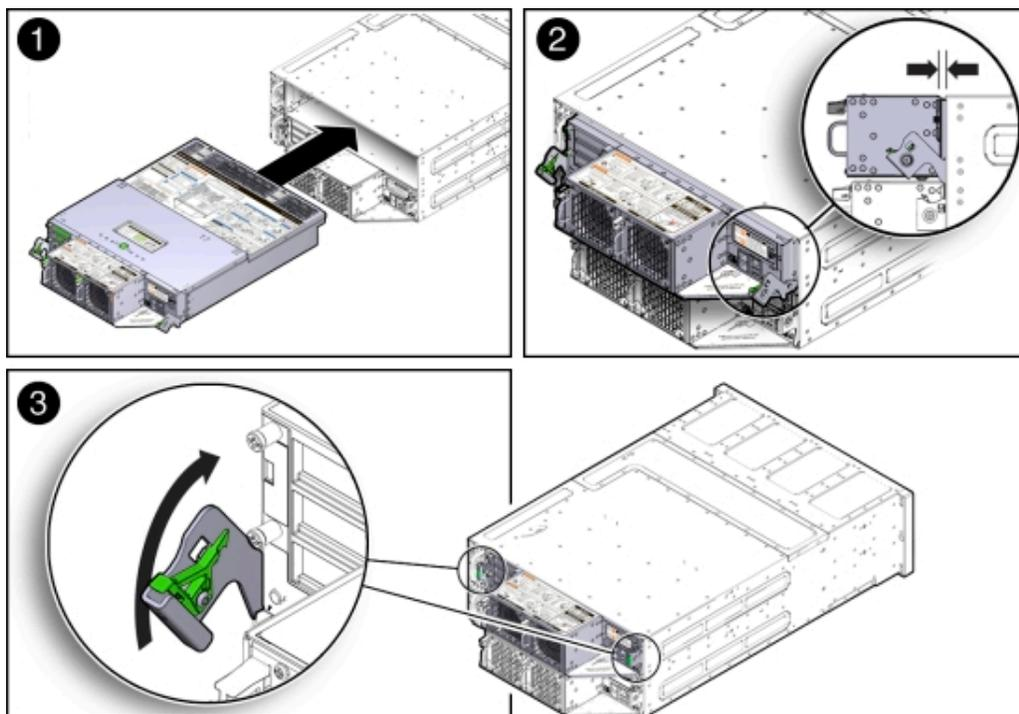
2. Slide the server node into the rear of the system chassis until the bottom lips of the release latches touch the chassis [2].
