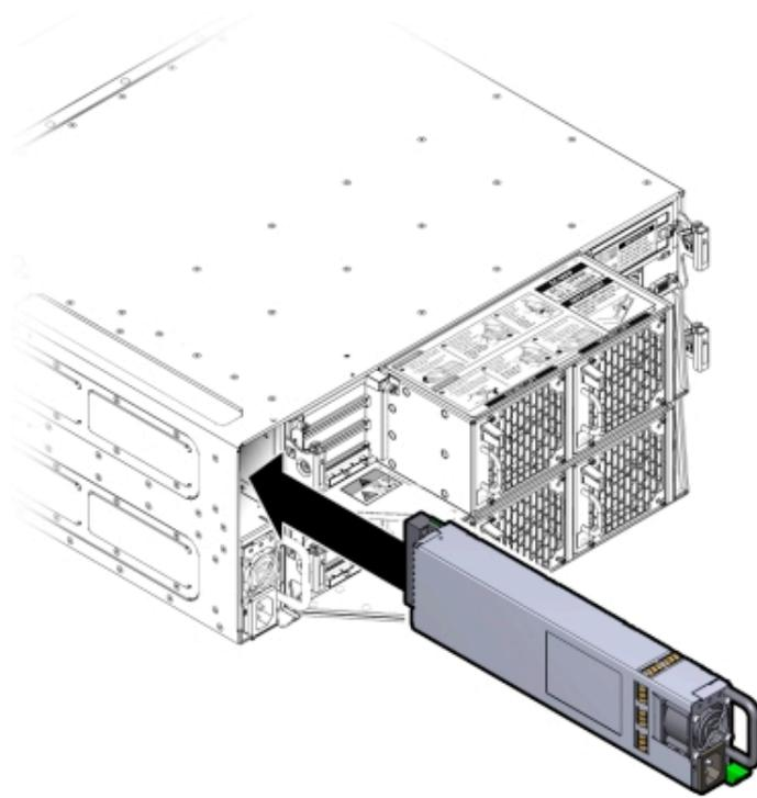
**3. Reconnect the power cord to the power supply and verify the following:**
