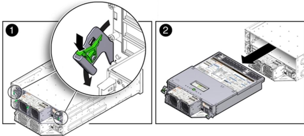
3. Slide the server node to the rear and lift it out of the system [2].
