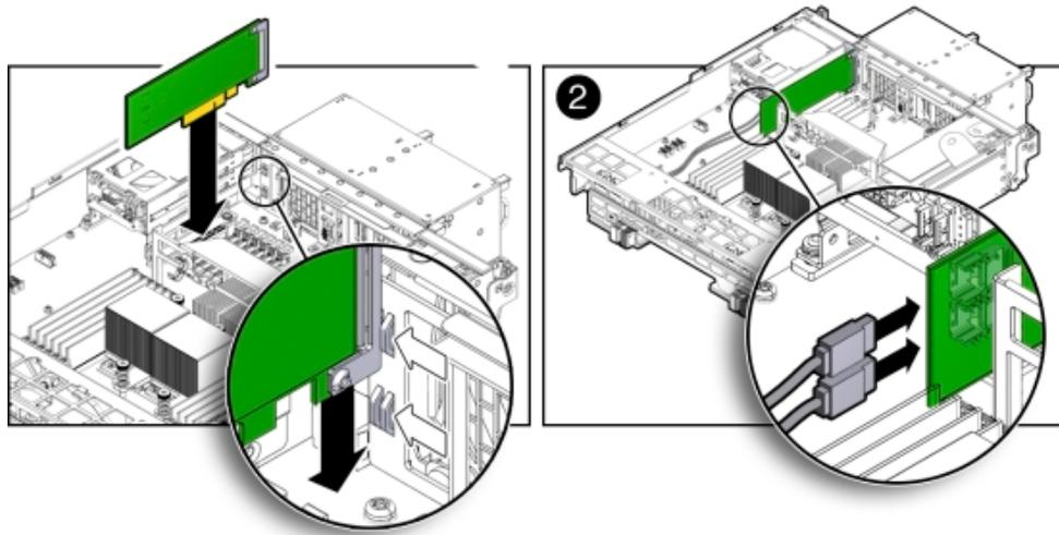
**b. Align the notch on the PCIe card with the key on the motherboard connector [1].****c. Align the rear of the PCIe card with the support bracket located on the rear of the server node [1].****d. Press down on the PCIe to seat it into the connector [1].**
