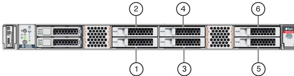
If you have the default configuration of only two NVMe drives (seen as `pd_00` and `pd_01` from the host), you can expand storage by either three (3) or six (6) NVMe drives.
