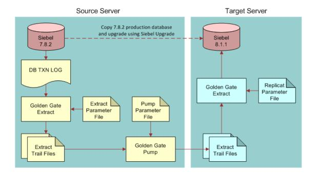
This figure shows two servers with Oracle GoldenGate software installed on each of them. Each server has a database instance: one is the source system Siebel CRM version 7.8.2, and the other has the target system, the current release of Siebel CRM. The directory structure and files reflect this environment.
