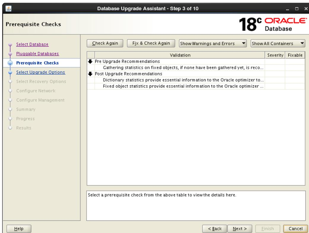
The Prerequisite Checks window shows the checks that DBUA has completed, and the severity of any errors discovered. When DBUA finds errors, it indicates which errors are fixable, and what action you can take to correct the error.
