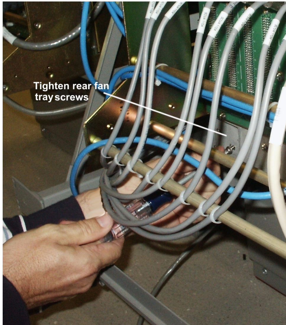
Figure 6-21 Tighten rear fan tray screws
