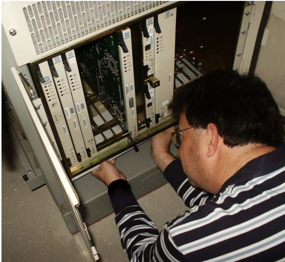
Figure 6-17 Insert fan tray bracket
