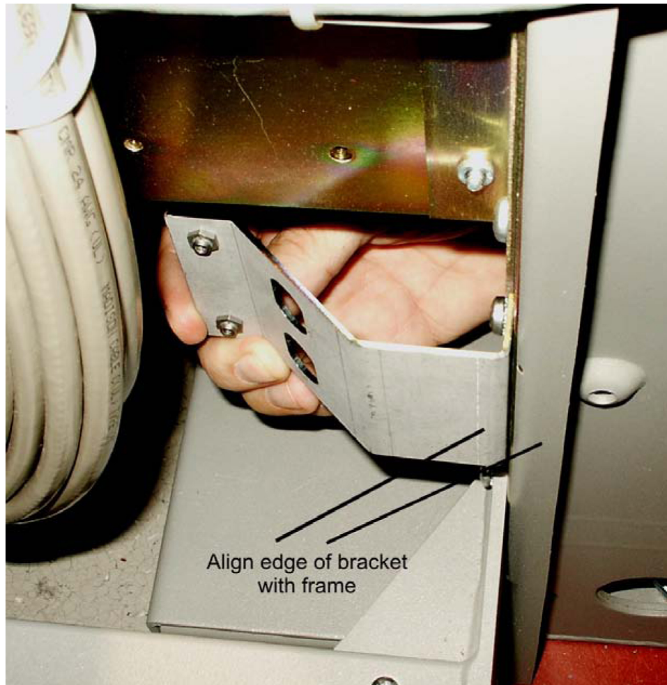
Figure 6-15 Slide the side fan brackets flush with the Frame
