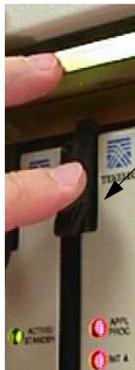
Figure 6-12 Push in Inject/Eject Clamps
