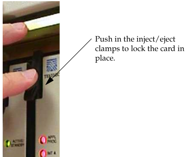
Figure A-12 Push in Inject/Eject Clamps
