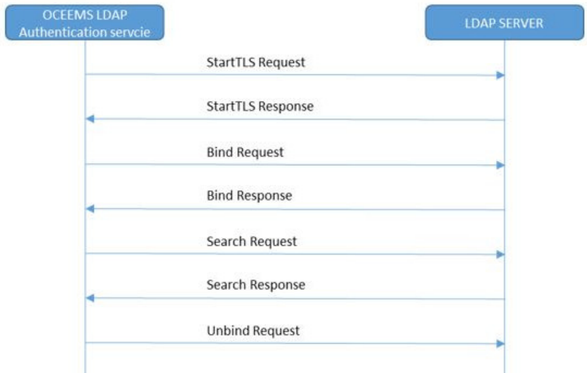
Figure 7-1 Sample Call Flow for LDAP Authentication
