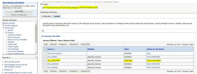
4. When all requested servers are running, goto deployments and check if deployments are in active state.
