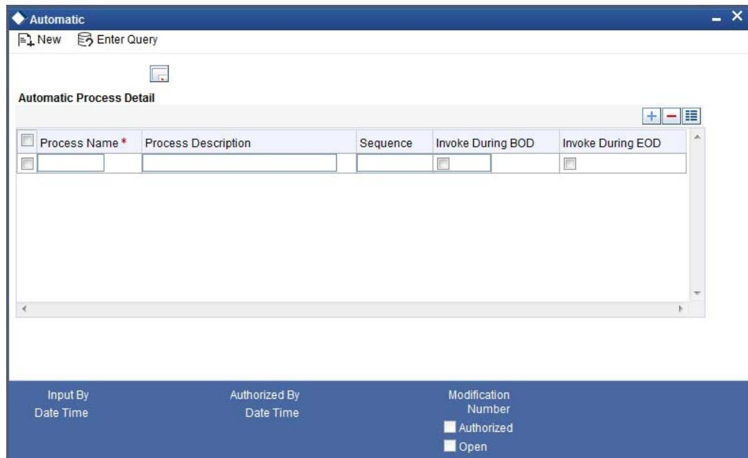
In this screen, you can amend the order of the various operations in the CL batch and choose to trigger them at EOD or BOD or both.
