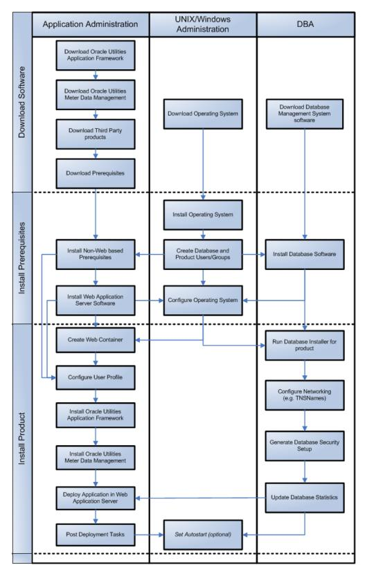
The following diagram provides an overview of the steps that need to be taken to install and configure Oracle Utilities Meter Data Management:
