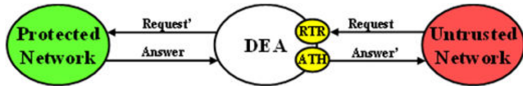
Figure 9-3 Diameter Topology Hiding Trigger Points: Untrusted-to-Protected Transactions
