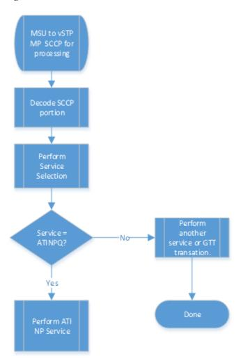
Figure 3-9 ATI NP Function Flow Chart - Sheet 1 of 3
