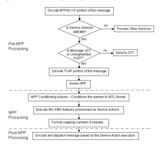
Figure 6-14 MO SMS NPP Message Processing
