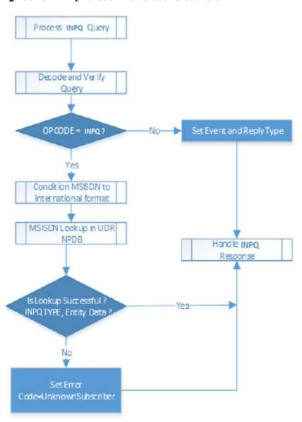
Figure 3-13 INPQ Function Flow Chart - Sheet 2 of 3
