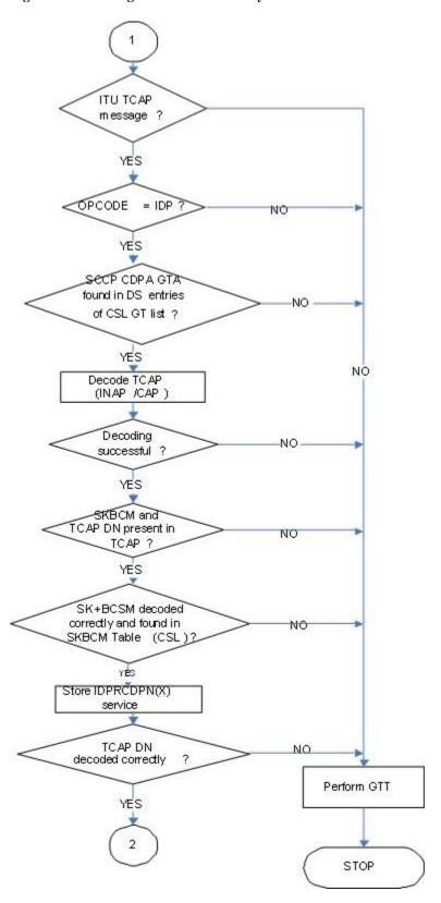
Figure 6-2 Message Flow for IDP Relay - Sheet 2 of 3
