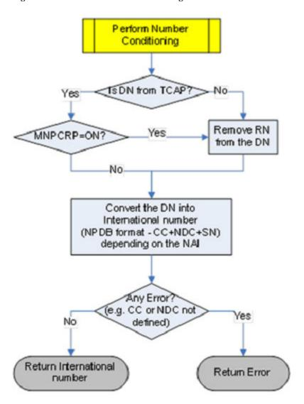
Figure 3-3 G-Port Number Conditioning Flowchart
