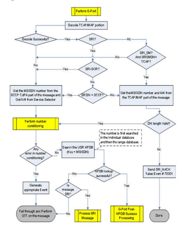
Figure 3-2 vSTP MNP G-Port Function Flowchart - Sheet 2 of 2
