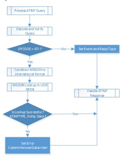
Figure 3-10 ATI NP Function Flow Chart - Sheet 2 of 3
