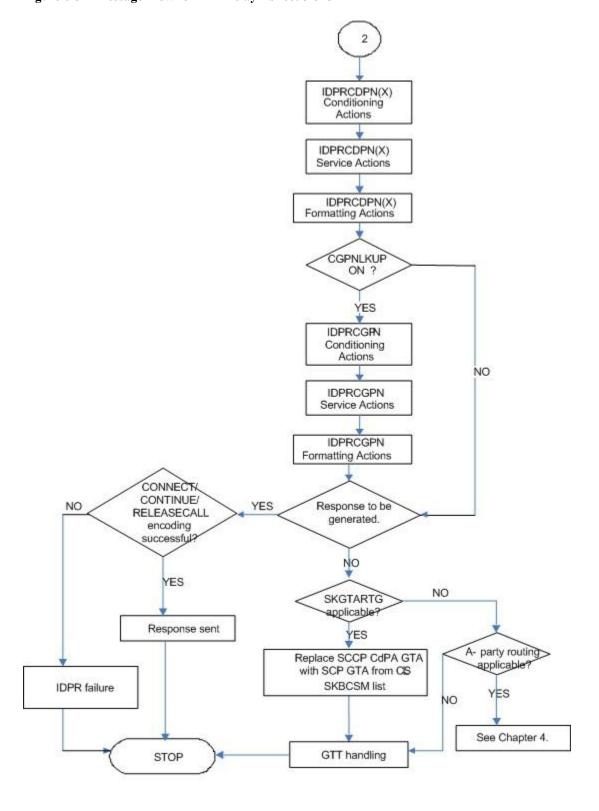
Figure 6-3 Message Flow for IDP Relay - Sheet 3 of 3
