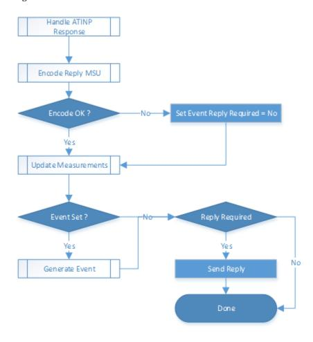
Figure 3-11 ATI NP Function Flow Chart - Sheet 2 of 3
