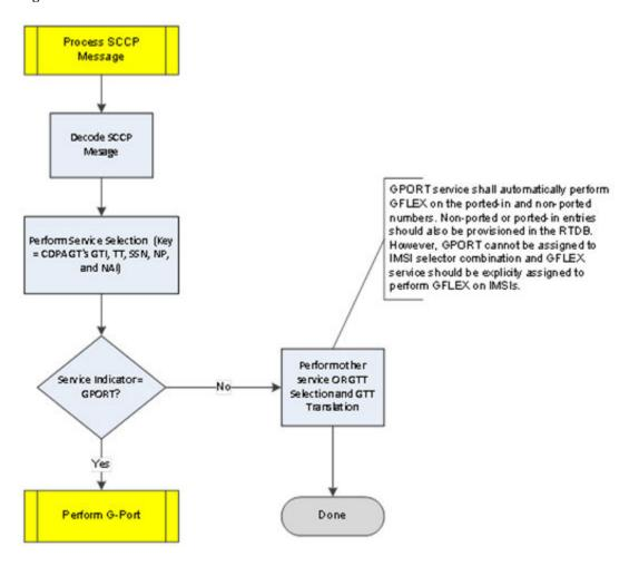
Figure 3-1 vSTP MNP G-Port Function Flowchart - Sheet 1 of 2
