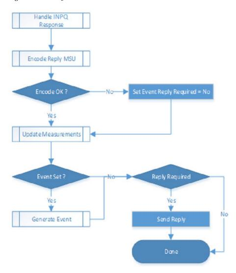
Figure 3-14 INPQ Function Flow Chart - Sheet 3 of 3
