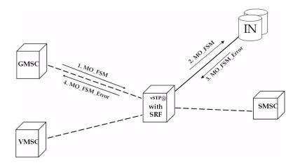
The Gateway Mobile Switching Center (GMSC) sends the Mobile Originated Forward Short Message (MO\_FSM) to the vSTP with PPSMS (TCBEGIN).
