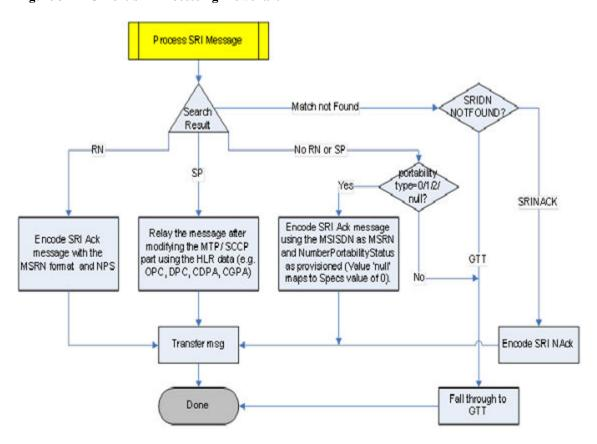
Figure 3-7 G-Port SRI Processing Flowchart
