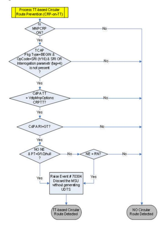
Figure 3-6 G-Port CRP on TT Flowchart
