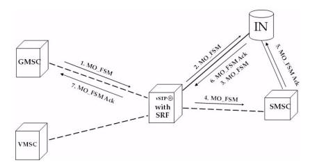
Figure 6-12 Successful Delivery of Mobile Originated FSM from Prepaid Subscriber
