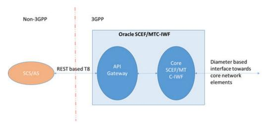
Figure 1-2 SCEF/MTC-IWF Functionality at DSR
