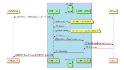
The UE sends a NAS message with EPS bearer ID and non-IP data to the MME. The MME/SGSN sends the NIDD Mobile Originated Data Request containing User Identity (IMSI), EPS Bearer Identifier, and non-IP data message to SCEF. When SCEF
