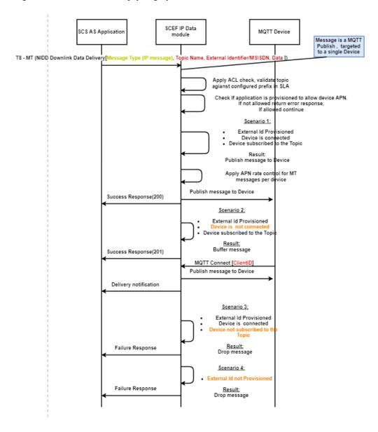
Figure 2-25 Data Delivery (Single) Call Flow
