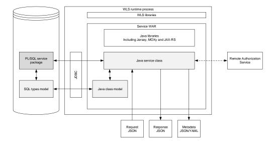
The high level schema below shows how the services are deployed. It also shows the database connection to OHI which uses a database account with restricted access to execute the HSL service implementation in PL/SQL.
