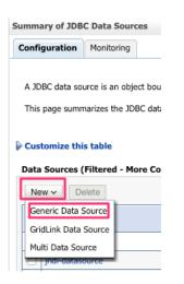
3. Enter a Name for the Data Source and a JNDI Name, and the database type. In the initial release of the RDC tool, 'Oracle' is the only supported Database type. In future releases this will be expanded to other vendors. Note – the JDNI Name forms part of the URL used to access the data source, so try to avoid spaces and other characters that may cause problems with the URL. Hit 'Next' to continue.
