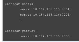
Here there are two load balancers defined. Default load balancing technique: **Round Robin** This block must be placed inside the http block.
