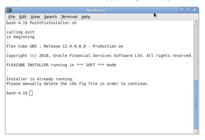
In this case, you have to delete the file 'chk.flg', that has been created in the installer sources and re-launch the Installer.
