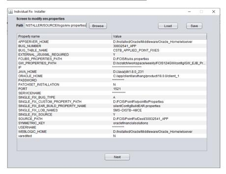
This is the screen where "env.properties" will be loaded from rolled up installer and user can edit the property file.
