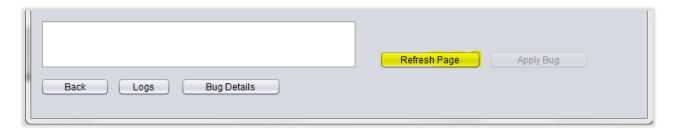
When a new zip file is added in the **Individual Fix Folder Path** and it needs to be listed in left side panel without relaunching installer, then **Refresh Page** button should be clicked.
