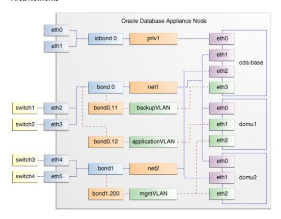
Figure 12-4 Oracle Database Appliance Virtualized Platform with Virtual Local Area Networks
