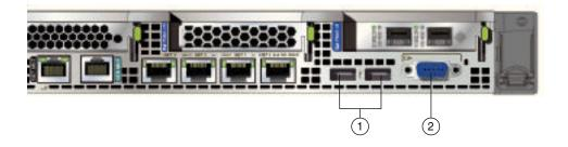
In the figure, callout 1 identifies the ports for the keyboard and mouse. Callout 2 identifies the monitor port.
