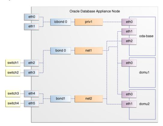
Figure 12-3 Basic Virtual Machine Local Area Network
