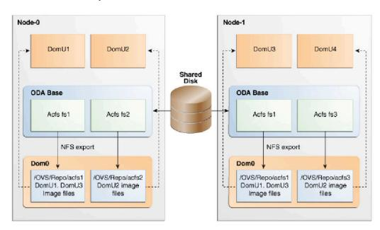
Figure 12-2 Architecture Overview of Oracle Database Appliance Virtualized Platform Shared Repositories
