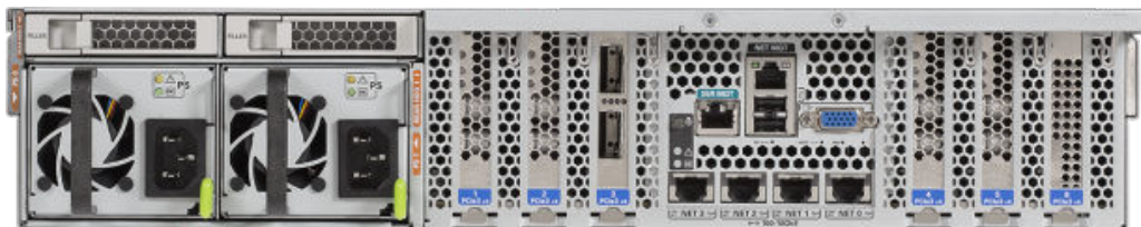
Figure A-36 Rear View of Exadata Storage Server X3-2L Servers
