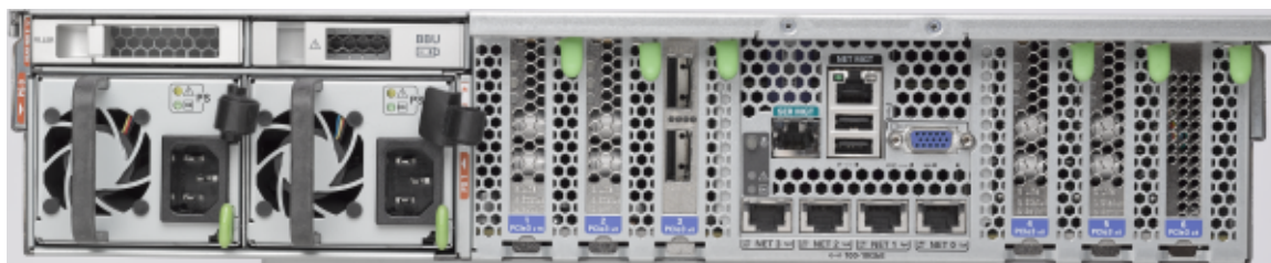
Figure A-34 Rear View of Exadata Storage Server X4-2L Servers
