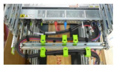
9. Secure the InfiniBand or TwinAx cables with hook and loop straps at equal intervals.
