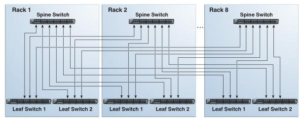
As shown in the preceding graphic, each leaf switch has eight inter-switch connections distributed over all spine switches. Each spine switch has 16 inter-switch connections distributed over all leaf switches. The leaf switches are not directly interconnected with other leaf switches, and the spine switches are not directly interconnected with the other spine switches.
