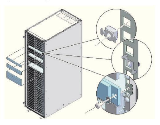
Figure 1-3 Removing the Filler Panels
