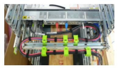
**8.** Connect the InfiniBand or TwinAx cables with the initial bend resting on the CMA. The TwinAx cables are for client access to the database servers.
