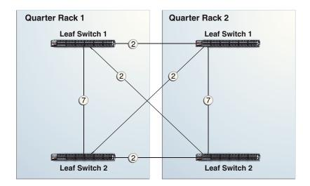
Figure 2-5 Leaf Switch Connections Between 2 Quarter Racks
