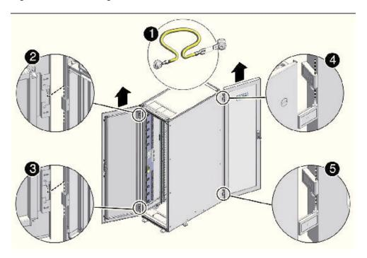
Figure 1-2 Removing the Rack Doors
