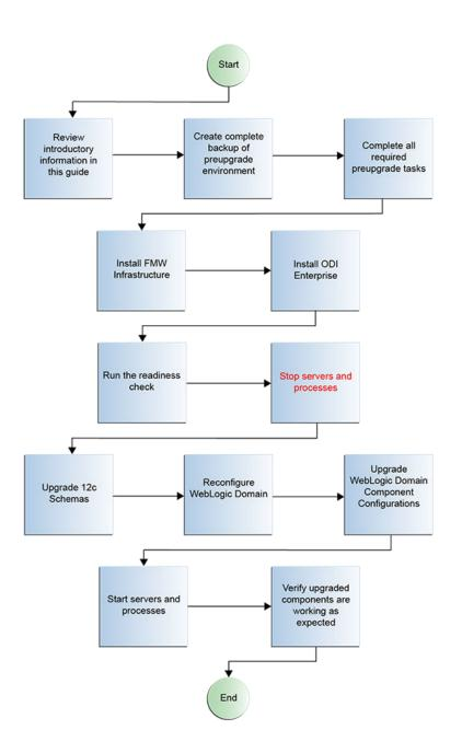
Figure 8-1 Oracle Data Integrator Java EE Agent Upgrade Process Flowchart
